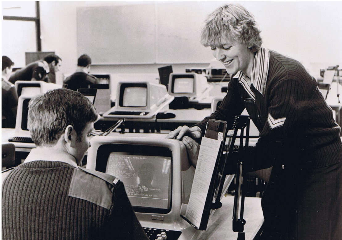
Part of the Poly installation for the Australian Army. Note the handles on the side of the Polys in the middle distance. These were to make it easy for children to carry machines between classrooms. They were dispensed with on the PolyCs.
